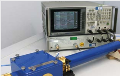
Coupling resistance, triaxial pipe
