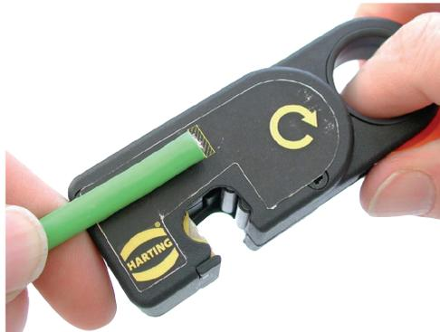
3. Insert the end of the cable into the tool and clamp it by activating the orange lever.
