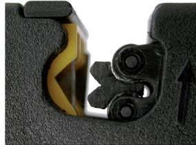
2. Measure the length of the cable according to the template on the right side of the tool. Place your left index finger against the front side of the tool as a limit stop.
